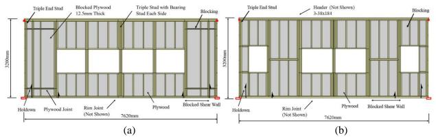
Figure 1. Exterior wall framing and configuration, north and south elevation: (a) Pattern "A", (b) Pattern "B".
