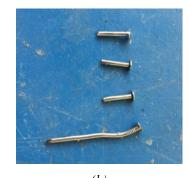
(a) (b) Figure 7.Damage in Specimen Sp-4 after test #2, a) North-east shear wall, b) Shear off nails.
