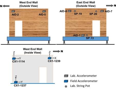
Figure 3. Instrumentation layout on the end walls of the specimen.
