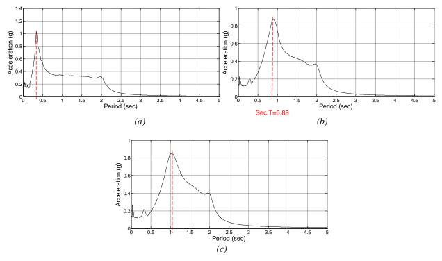
*Figure 10. Sine sweep acceleration response spectrum from Specimen Sp-6: a) Sine Sweep 1, b) Sine Sweep 2, c) Sine Sweep3.*
