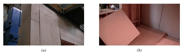
*Figure 6. Damage in Specimen Sp-1 after test # 3: a) Southwest shear wall, b) Internal view of drywall.*
