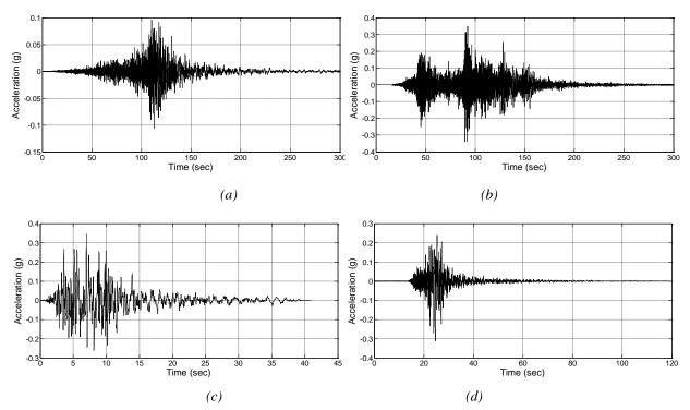
Figure 4. Acceleration time history records for testing program (100% amplitude): a) Tohoku SIT002 station, b) Tohoku MYG016 station, c) Kobe KAK station, d) Geiyo EHM008 station.
