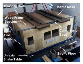
Figure 2. General view of the test setup for shake table testing
